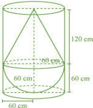
Radius ( $r$ ) of hemispherical part = Radius ( $r$ ) of conical part = 60 cm
