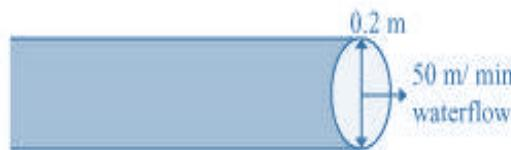
Consider an area of cross-section of pipe as shown in the figure.
