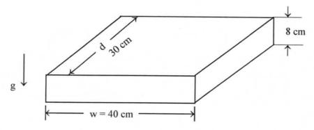
The top surface of the case has to dissipate 25W to the surrounding air, which is at 20°C. The emissivity of the surface is 0.6. Determine the temperature of the top surface, Given  $\beta$ =3.411×10<sup>-3</sup>/K.
