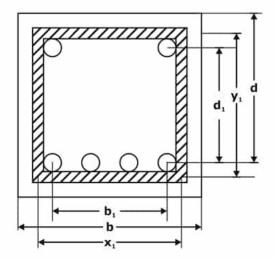
$x_1 = b_1 + Diameter of longitudinal bar + Diameter of stirrup$
