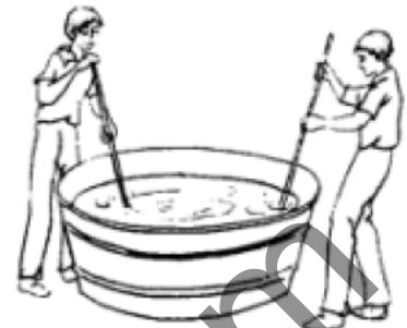
(b) Scouring in tanks
